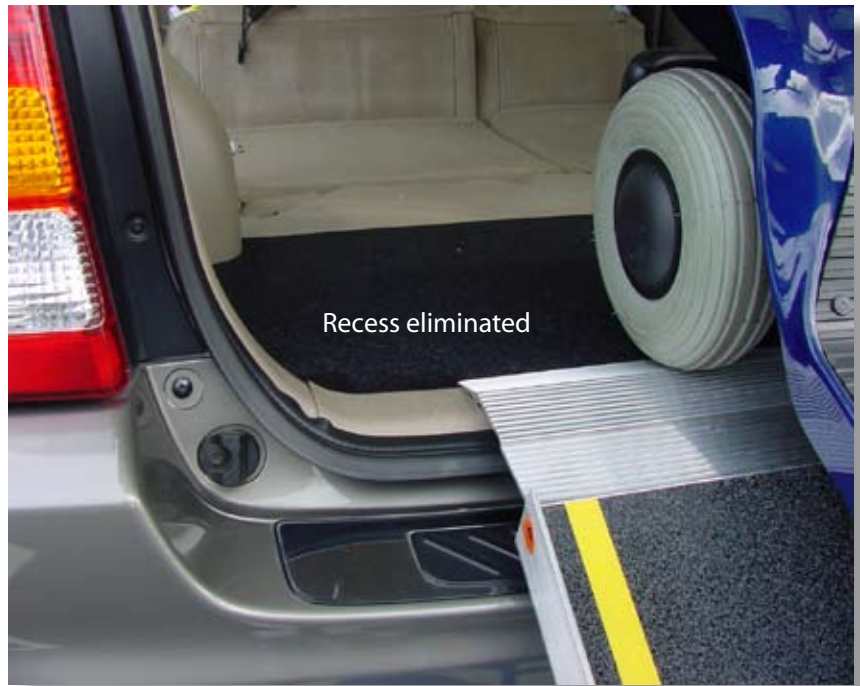
CARGO WEDGE shown with an Advantage Series SUITCASE ramp with the TLE option
